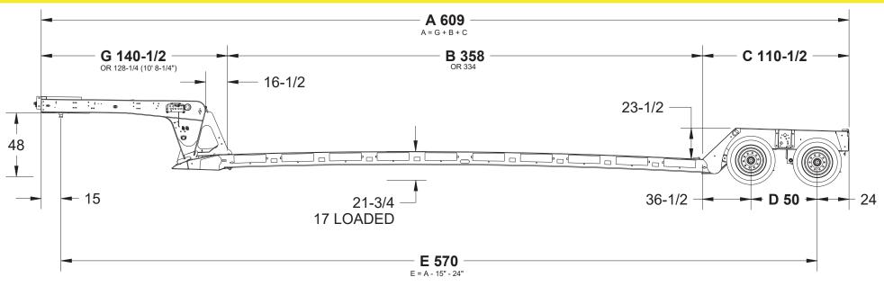
MODEL. # OF AXLES. **AXLE SPREAD TOTAL LENGTH** GOOSENECK (G/N) L/D BED LENGTH 825 AG 2AX 50SPD SHOWN 609 (50' 9") 140-1/2 (11' 8-1/2") 358 (29' 10") 825 AG 2AX 50SPD 334 (27' 10") 585 (48' 9") 140-1/2 (11' 8-1/2") AX = AXLESPD = SPREAD 825 AG 2AX 50SPD 596-3/4 (49' 8-3/4") 358 (29' 10") 128-1/4 (10' 8-1/4")
